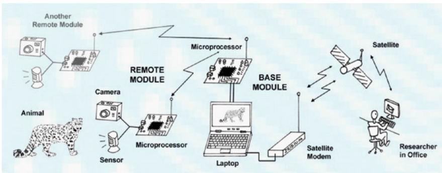
**Fig. 3.1** Prototype satellite linked, wireless camera trap network (C. Bray, pers. commun.; <http://scoff.ee.unsw.edu.au/posters/posters2006/Satellite%20Linked,%20Wireless%20Camera%20Trap%20Network.pdf>)
