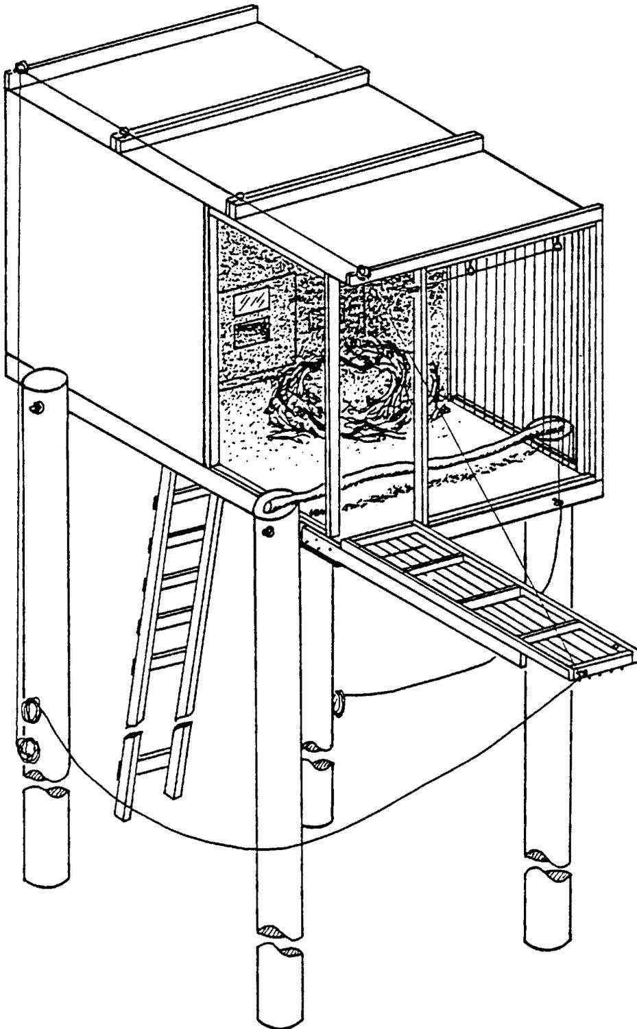
Figure 2. Diagram of a Bald Eagle Hacking Platform with Cut-away View of Nest Area. The Fledging Door is Shown in the Lowered Position. Fledging Door was Lowered By Ropes From Behind the Platform.
