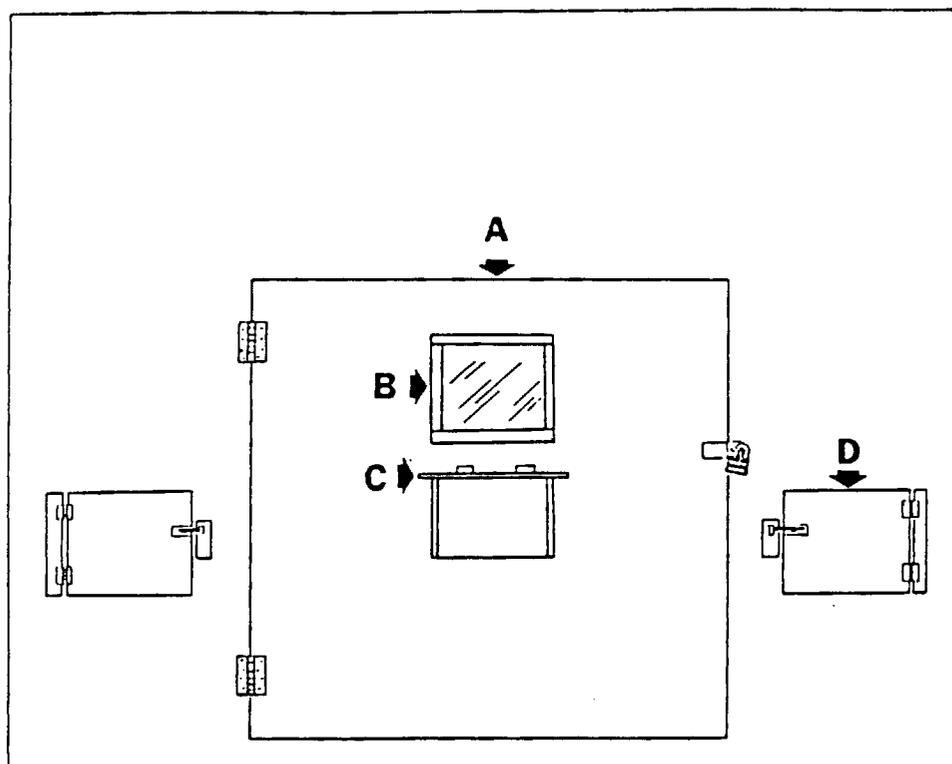
Figure 4. Diagram of the Wall Separating the Blind From the Nest Area on the Hacking Platform. A) Door Which Allows Access to Nest Area; B) One-Way Glass for Viewing the Birds; C) Surface for Note Taking; and D) One of Two Food Access Doors for Introducing Food.
