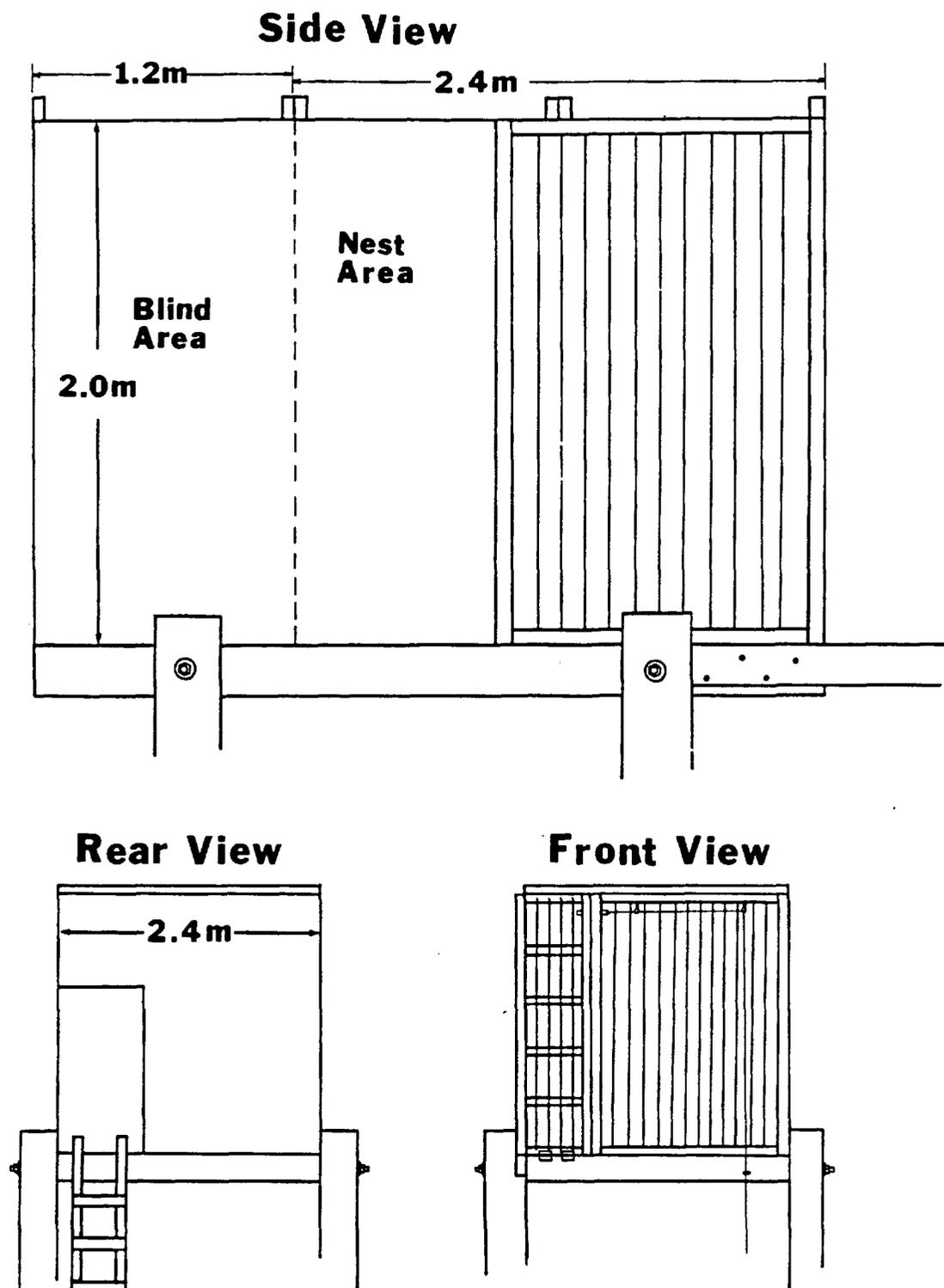
Figure 3. Views of a Hacking Platform: Side View, Showing Barred and Plywood (Solid) Portions of the Nest Area, and the Blind Area; Rear View, Showing Ladder Access to the Blind; and Front View, Showing Release Door (Left Side) and Bars.
