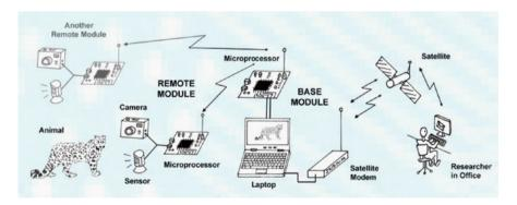
**Fig. 3.1** Prototype satellite linked, wireless camera trap network (C. Bray, pers. commun.; http://scoff.ee.unsw.edu.au/posters/posters2006/Satellite%20Linked,%20Wireless%20Camera%20Trap%20Network.pdf)
